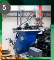
Harfield tableware is sorted, ground down, ready to be reused. The recycled tableware is then remoulded into non food contact products.
